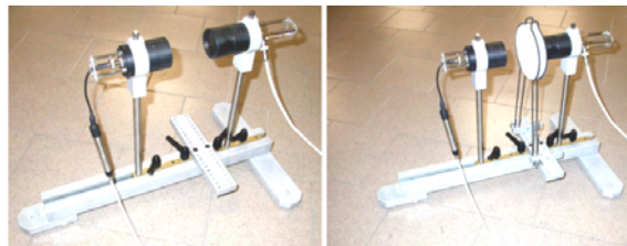
Experimental set-up for measuring tortuosity
